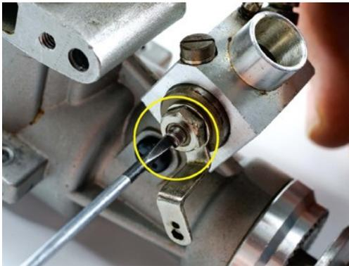
**To adjust the low-end needle valve, you have to use a fine tip screwdriver. For safety's sake, be sure to stop the engine before you adjust it.**
