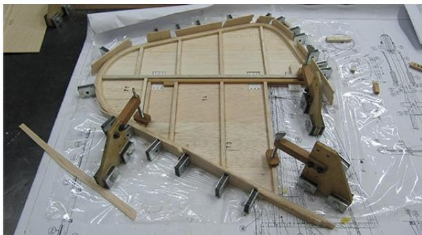
In the left photo, the bare magnets are used to hold the 4 laminated strips of wood securely to the building board and Piper Cub vertical stabilizer/rudder assembly to form the leading and trailing edges.
